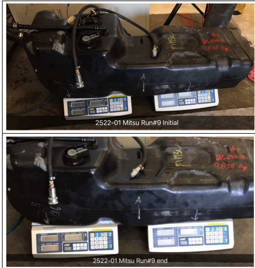
Figure 8. Initial auxiliary tank weighing following refuel (Top) and ending auxiliary tank weighing following a circuit run (Bottom).
