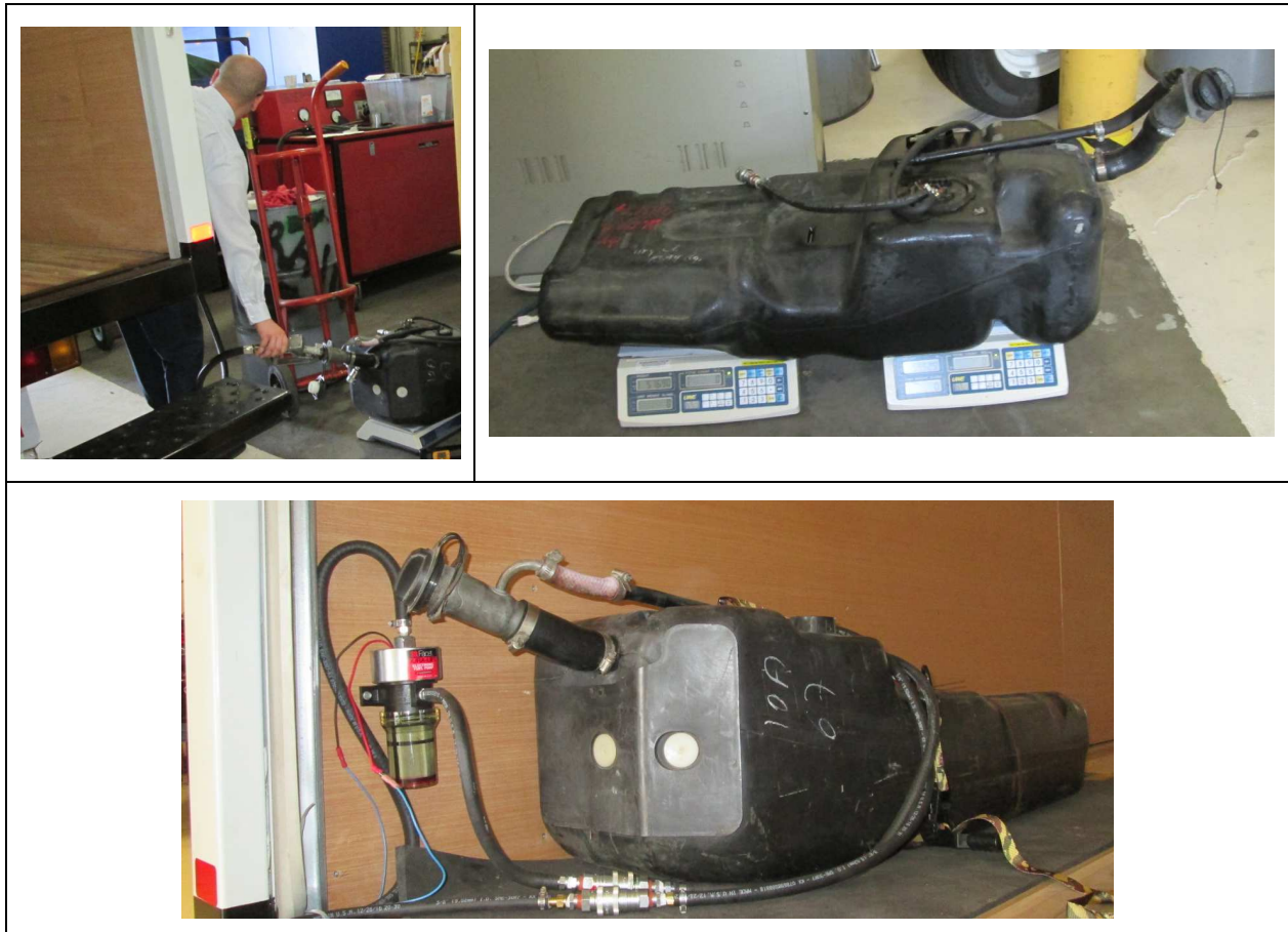
Figure 6. Refueling auxiliary fuel tank (Top Left), weighing auxiliary fuel tank (Top Right), securely mounting and reconnecting auxiliary fuel tank in box of truck (Bottom).
